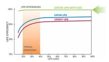
**ESS enables market-leading 99 percent efficiency** across the entire operating range. Compared to conventional 'eco-mode' capabilities available with legacy products, ESS offers the best possible efficiency and the fastest transition times to double conversion when power disturbances occur.
