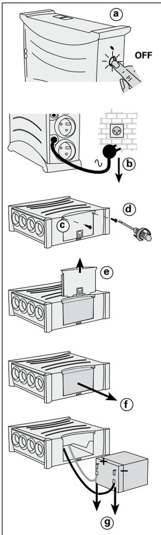
► **Warning:** take care not to invert the polarity + (red) and - (black) when connecting the batteries as this will destroy the device.
