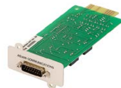
BD relay card (для ИБП Eaton 9130)
