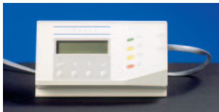
ViewUPS for remote monitoring and configuration
